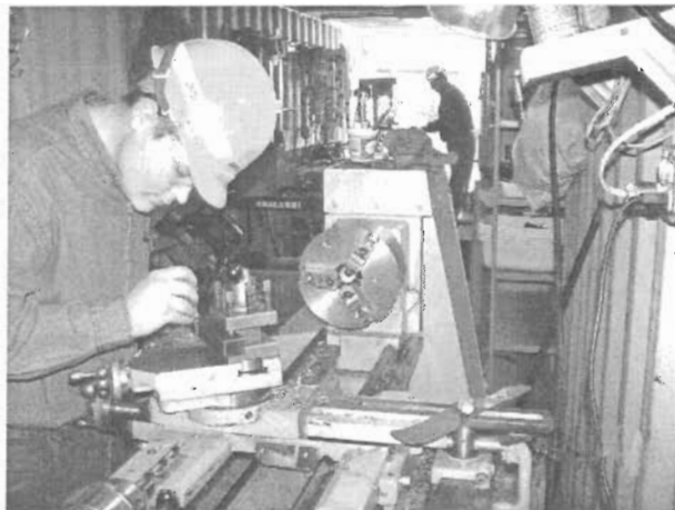
Atwell sets up the lathe to machine a part to replace one that was too rusty to reinstall on the tender. Chief Safety Officer Spargo is at the drill press in the background.
