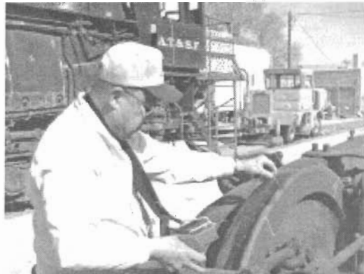
John Gieske focuses intently on the instrument display as he moves the sensor slowly over the face of the wheel. The ultrasound instrument can detect flaws deep inside the wheel.
