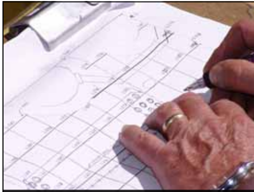
All measurements derived from ultrasound readings were carefully entered into charts drawn to represent a specific portion of the boiler.
